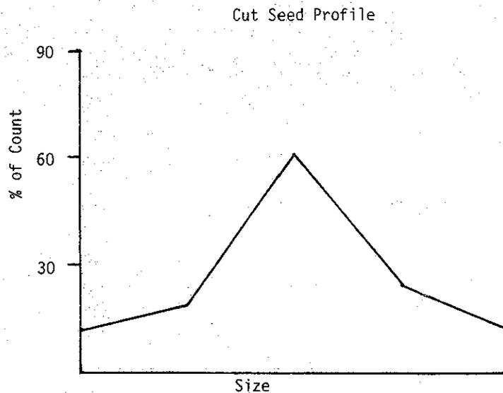
The third input necessary is the placement of the seed in the field by the planter. A standardized area behind the planter is measured and the seed is uncovered. The location of each seed is recorded on a form and the data used to calculate the accuracy of the planter. A graph can be drawn which shows the planter's performance over a period of time. (Fig. 3).
