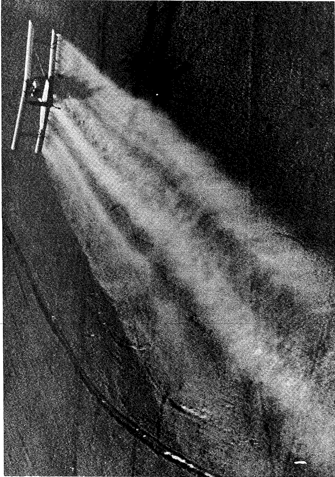
Streaked spray pattern from improperly placed nozzles
