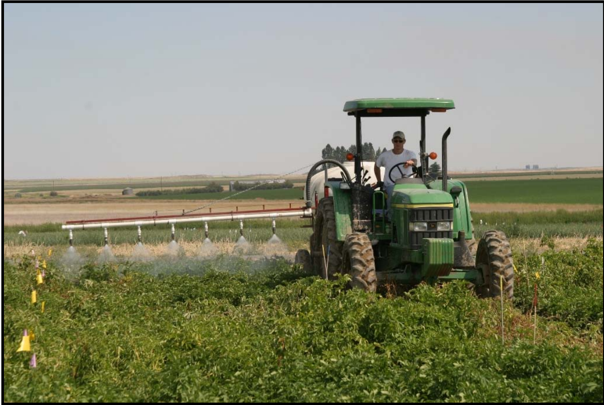
Figure 1. Chemigation simulation unit applying in-season fertilizer treatments on the Othello Research station.
