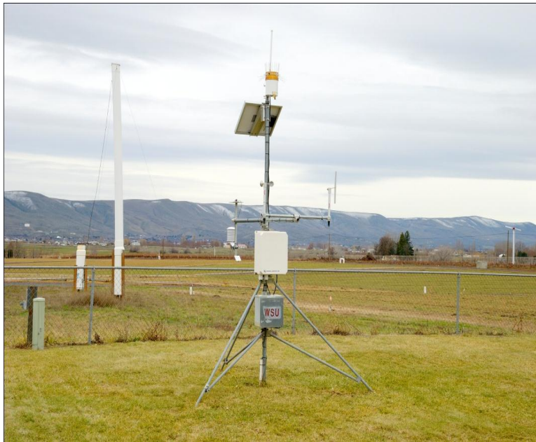
Figure 2. Automated weather station at the Irrigated Agriculture Research and Extension Center (IAREC) in Prosser, Washington.
