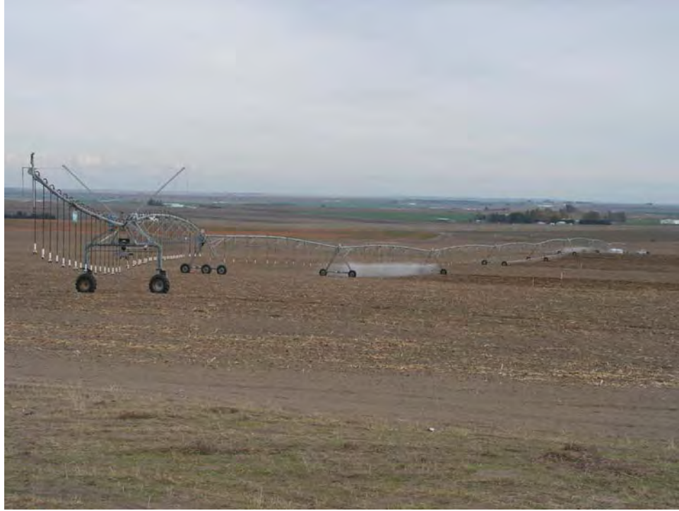
Figure 2: Sectagon 42 Center Pivot Water Run-Drizzle Boom Application
