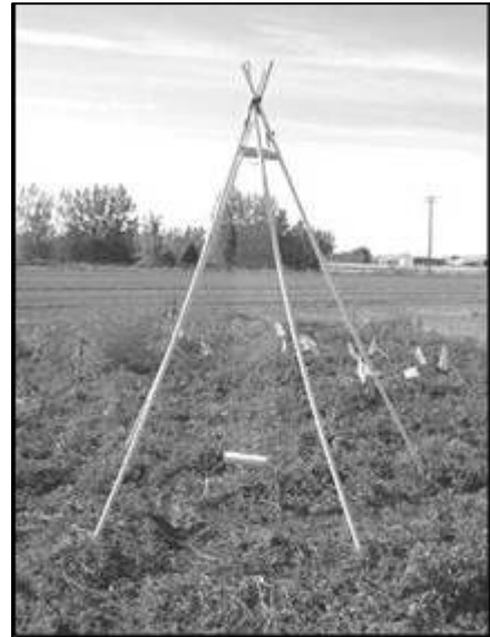
Figure 3. A teepee trap consisting of 3 pieces of 10' PVC and the net staked to the ground (see text).
